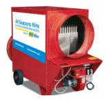
JUMBO space heaters have been designed for use in small to medium-sized rooms and buildings where a fixed or mobile heating system is required. Heat is produced by combustion and the heat from the smoke is transmitted to the fresh air through the metal walls of the combustion chamber and the heat exchanger. The combustion chamber is of the type where smoke circulates twice.
