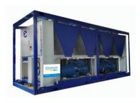
The 500kW chillers is the second largest individual unit in the All Seasons Hire range. With dual refrigerant circuits there is resilience built in, with the chiller able to continue operation with a fault on one circuit. Despite this units overall size the sturdy steel constructed frame enables easy listing and positioning with 6 lifting points and fork lift pockets.
